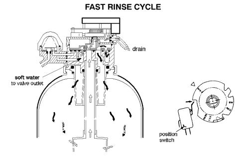
During FAST RINSE, the rotor & disc is positioned so water flow enters the resin tank through the top distributor, and exits through the bottom distributor, to the drain.
